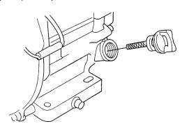
Figure 3. Engine Oil Dipstick
